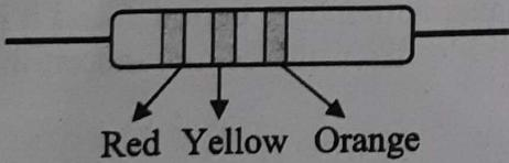
A carbon resistor with colour code is shown in the figure. There is no fourth band in the resistor. The value of the resistance is
