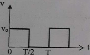
The rms value of potential difference v shown in the figure is
