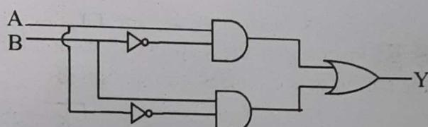
For the given logic circuit, the output Y for inputs ( $A = 0, B = 1$ ) and ( $A = 0, B = 0$ ) respectively are
