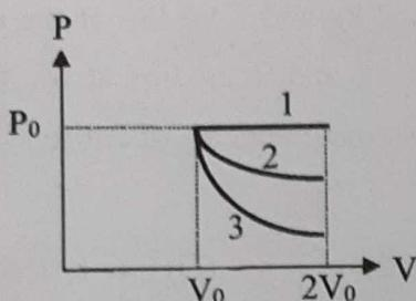
In the given figure, 1 represents isobaric, 2 represents isothermal and 3 represents adiabatic processes of an ideal gas. If  $\Delta U_1$ ,  $\Delta U_2$ ,  $\Delta U_3$  be the changes in internal energy in these processes respectively, then
